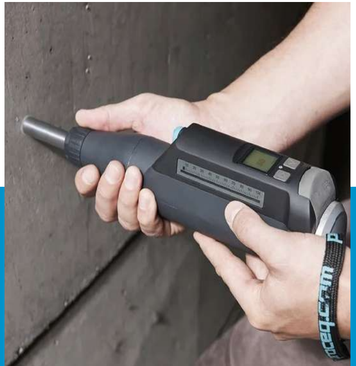
Rebound Hammer Test
