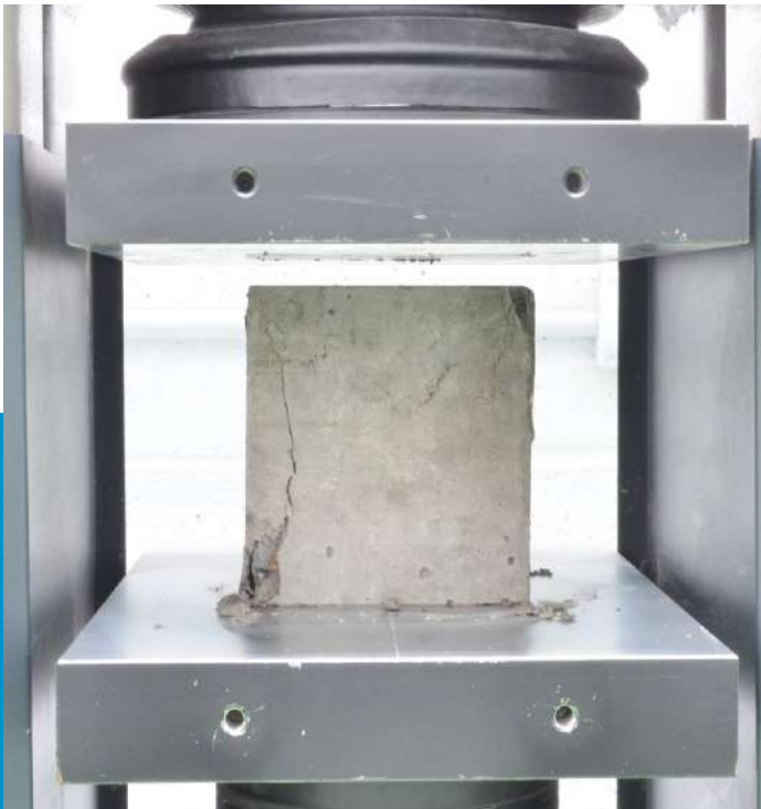
Concrete Strength Test
