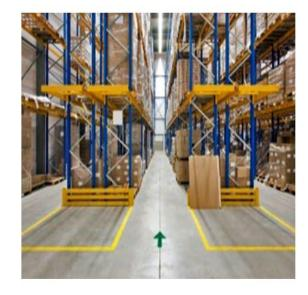
We provide service of VNA wire guidance system installation for very narrow aisle (VNA) trucks and Automated guided vehicles (AGV's). Installation of wire and transponders or magnets should be done very precisely because the sensors installed in the vehicle receives the signals from the wire embedded in the floor and system locks the steering when the vehicle is moving in the aisle.
